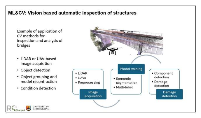
CV methods are increasingly applied to inspection and analysis, leveraging advanced technologies for comprehensive evaluations. LiDAR or UAV-based image acquisition captures high-resolution data of
