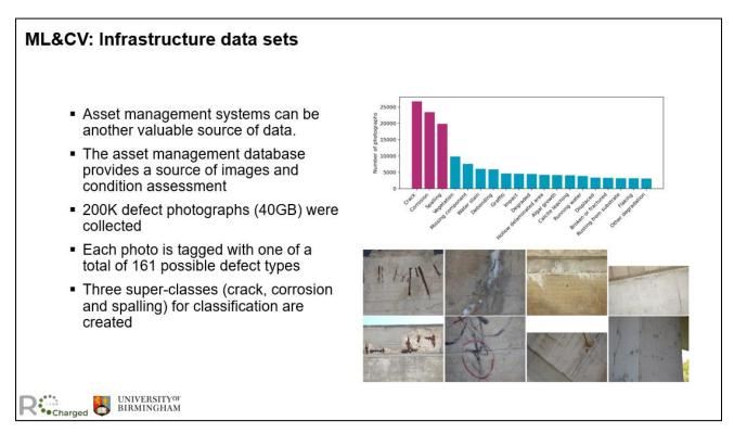
Asset management systems are crucial data sources for infrastructure management. For instance, the asset management database (Bush et al., 2021) offers extensive image and condition assessment data. The sown sample includes 200,000 defect photographs (Mundt et al., 2019), amounting to 40GB of
