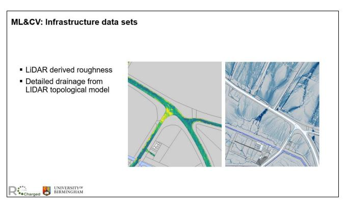
Pavement datasets include LiDAR-derived roughness measurements (Corker et al., 2023), which assess surface irregularities, and detailed drainage information from LiDAR topological models. These datasets provide critical insights into pavement conditions and drainage patterns, aiding in accurate assessment and effective maintenance, planning, and road infrastructure.
