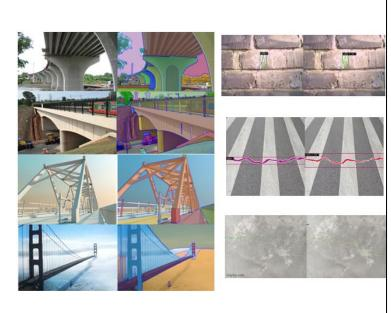
SAMcan detect bridge components by segmenting images into distinct regions, identifying and classifying parts like beams, joints, and cables. This enables precise analysis and monitoring of bridge infrastructure through detailed, component-level segmentation.
