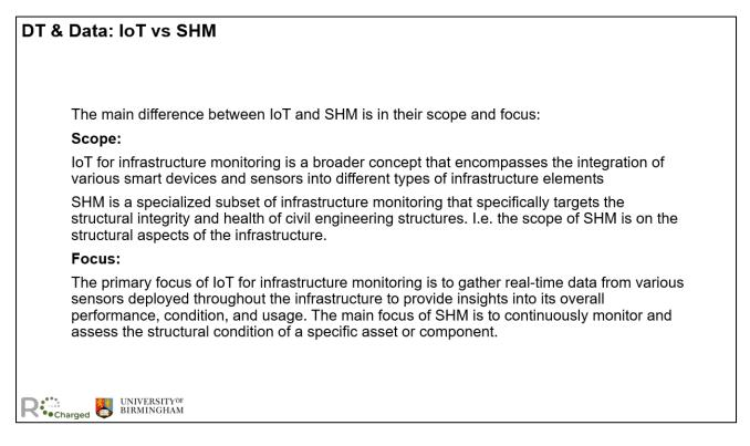
The main difference between IoT and Structural Health Monitoring (SHM) lies in their scope and focus. IoT for infrastructure monitoring is a broader concept that involves integrating various smart devices and sensors into different types of infrastructure elements. This allows for the collection of real-time data, providing comprehensive insights into the overall performance, condition, and usage of the infrastructure.
