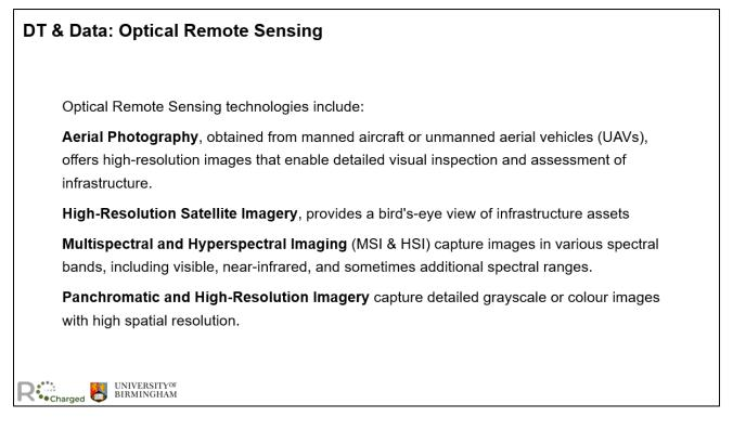
Optical remote sensing technologies are invaluable for infrastructure inspection and assessment. Aerial photography, whether from manned aircraft or UAVs, delivers high-resolution images for detailed visual inspections. High-resolution satellite imagery offers a comprehensive bird's-eye view of infrastructure assets, enhancing large-scale monitoring.
