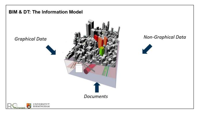
A BIM model integrates graphical data (3D visual representations of building elements), non-graphical data (attributes like material properties, costs, and performance metrics), and documents (such as drawings, specifications, and reports). This comprehensive combination provides a holistic view of the asset for effective management and analysis.
