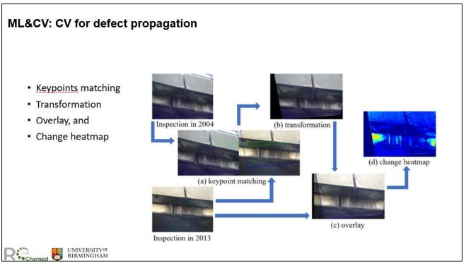
This helps in monitoring the progression of defects or damages over time (Bush et al., 2022). Tracking defect propagation involves several steps: key point matching aligns features across images, transformation adjusts for perspective changes, and overlay superimposes images to compare defect locations. Change heatmaps visualize and quantify defect growth, highlighting areas of increased damage over time for effective monitoring and analysis.
