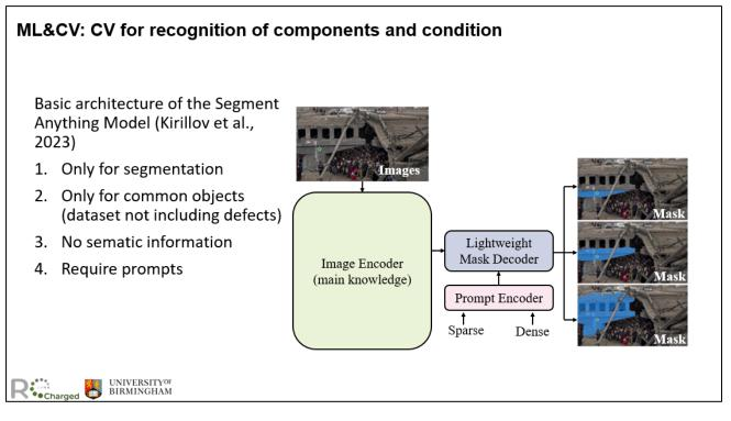
Traditional visual inspections of structural surface defects are labour-intensive, time-consuming, and subjective. Therefore, automation is crucial for increasing productivity. Basic architecture of SAM (Kirillov et al., 2023) is here; however, SAM can only do segmentation and only for common objects not for our tasks, no sematic information, and requires prompt to let model carry out. So, our aim is to propose an automatically framework for structural surface defect detection based on SAM.
