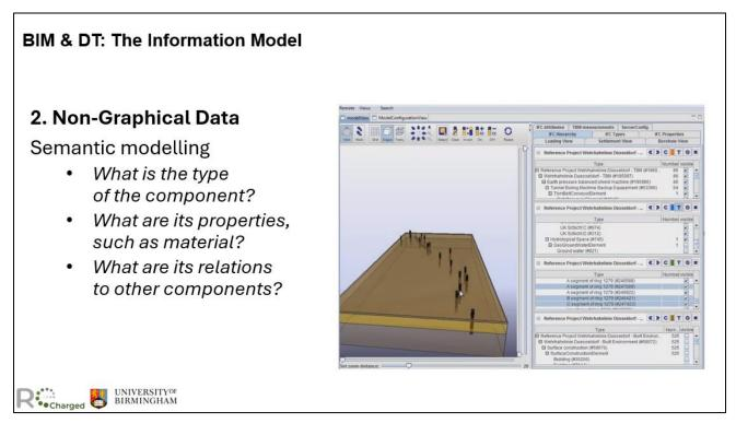
Non-Graphical Data in BIM (Koch et al., 2017) focuses on semantic modeling, which involves defining the type of each component and its properties, such as material. It also examines the relationships
